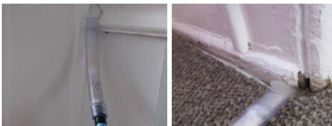
Figure 6 Smoke drawn behind end of dado detail and at bottom of window reveal
