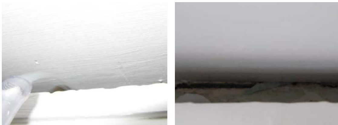
Figure 5 Smoke drawn over top of windows. Gaps visible above windows.
