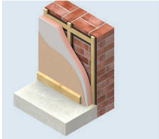
Diagram of internal wall insulation on battens
