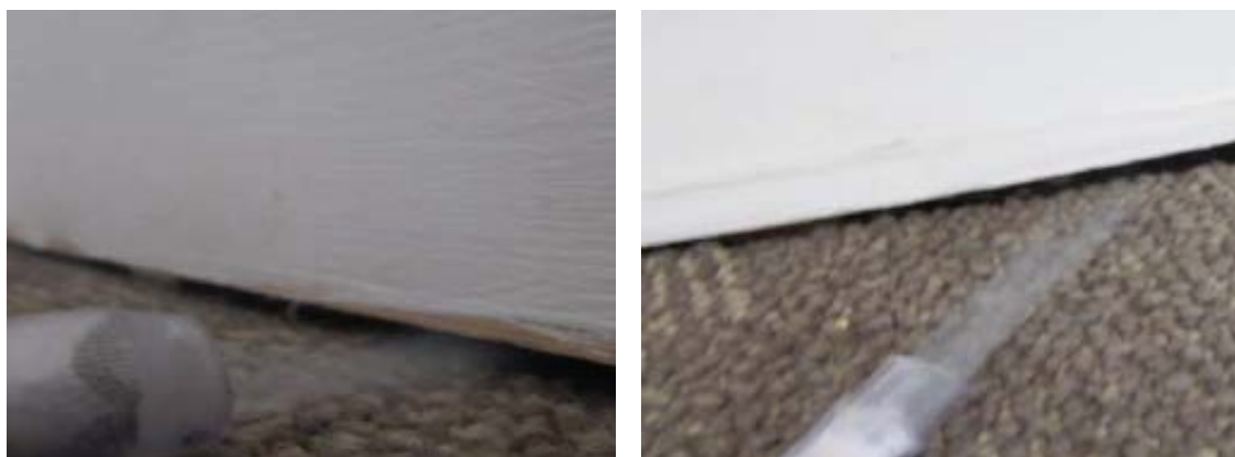
Figure 4 Smoke drawn through gap between floor and skirtings.
